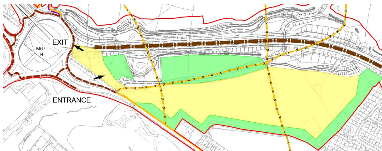
Figure 2.2: Site Compound (extract from 2.8 Temporary Works Plan)
